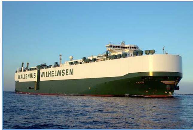
M/S Faust, a PCTC operated by Wallenius Wilhelmsen (capacity: 8000 CEU, LOA: 228m, beam: 33m, draft: 11.5m)
