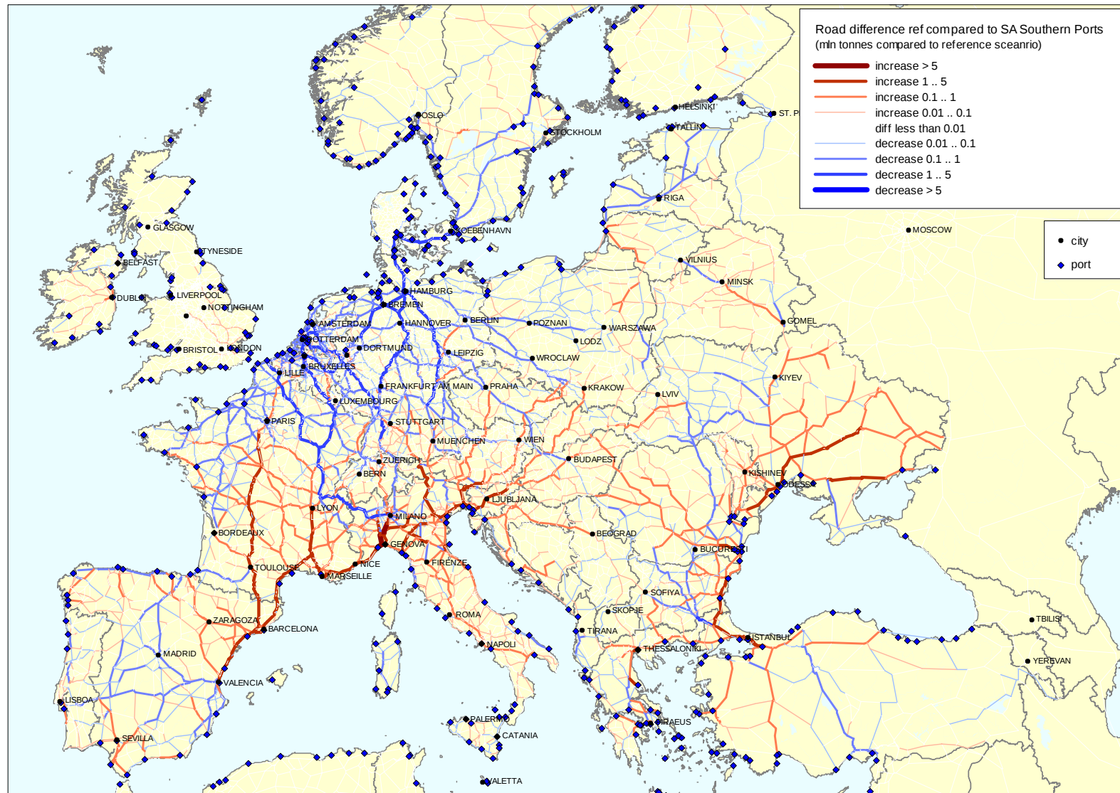
Figure 6.22 Comparison between 2030 North to South Sensitivity Analysis and Central Scenario, Road Transport
