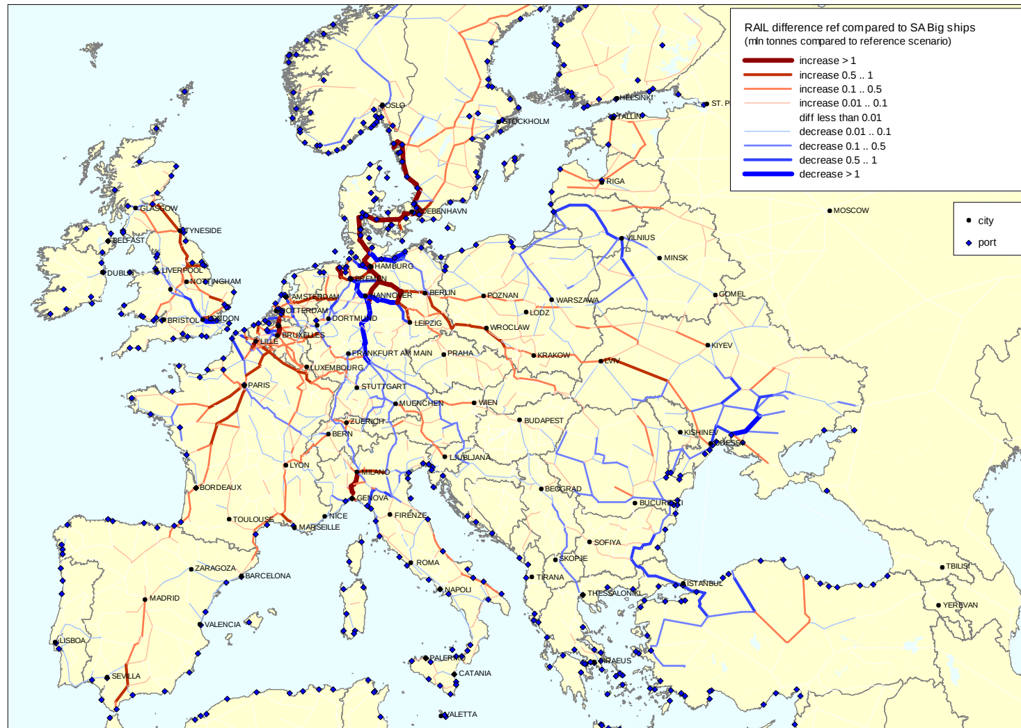
Figure 6.20 Comparison between 2030 Large Ships Sensitivity Analysis and Central Scenario, Rail Transport
