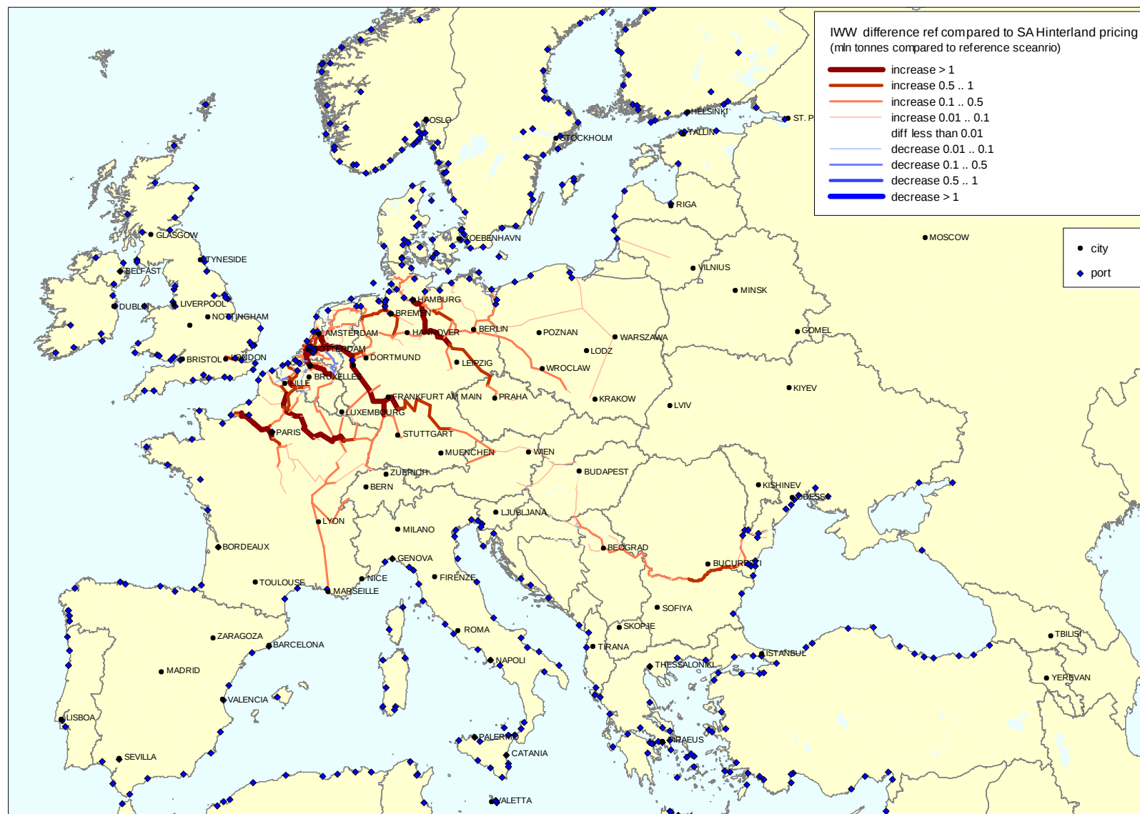
Figure 6.27 Comparison between 2030 Hinterland Pricing Sensitivity Analysis and Central Scenario, Waterway Transport
