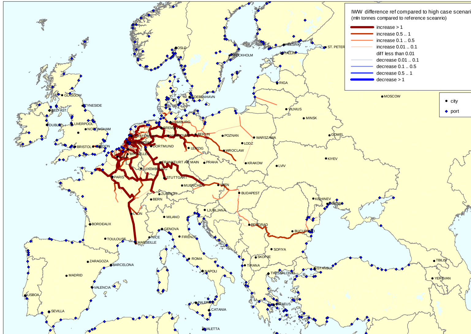
Figure 6.18 Comparison between 2030 High Case and Central Scenario, Waterway Transport
