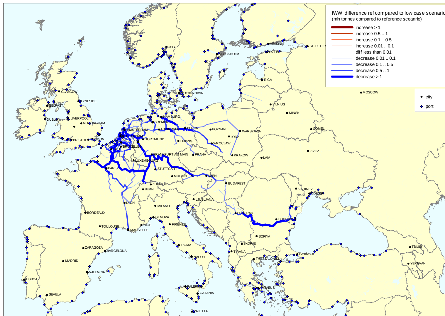
Figure 6.15 Comparison between 2030 Low Case and Central Scenario, Rail Transport
