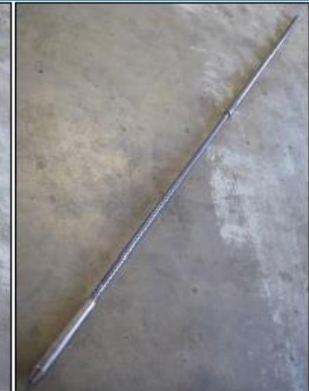
Bottom-up injection tool with retracted sheath
