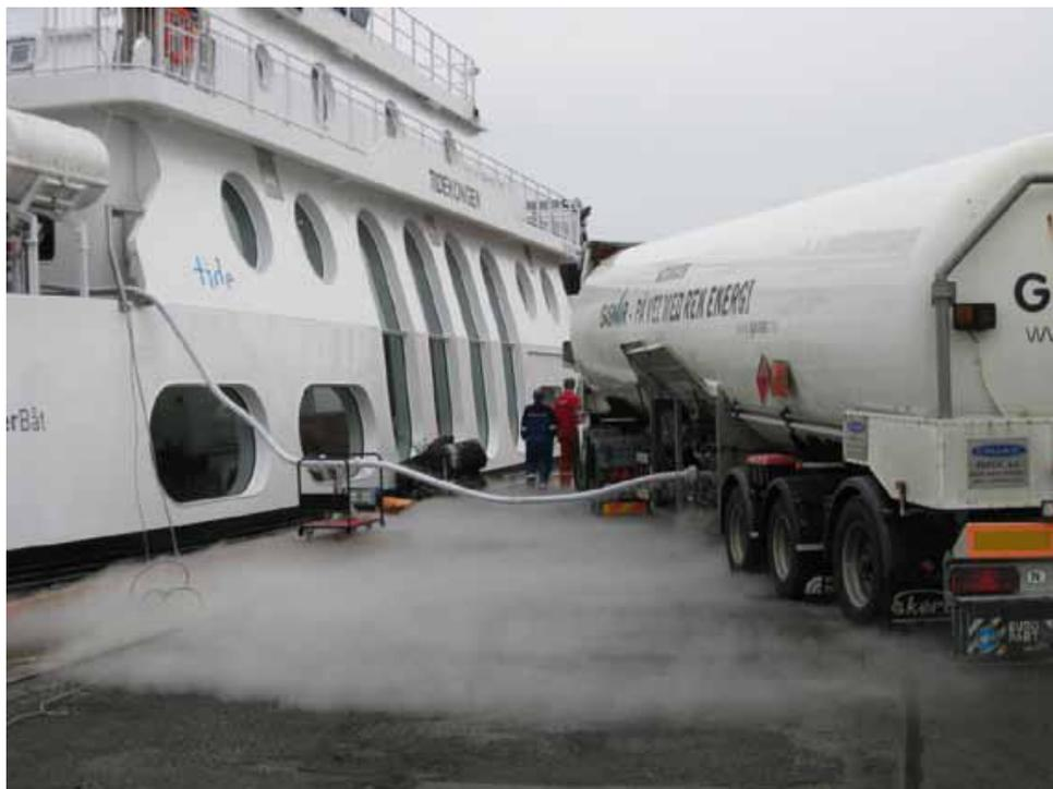
**Figura 16 - Rifornimento GNL Truck-To-Ship (TTS)**
