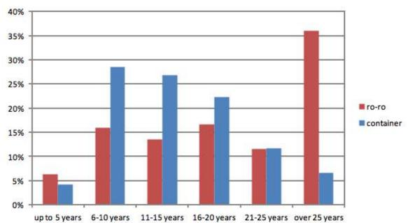
Figure 9: Age structure of the ro-ro and container fleet employed on regular European short sea services (spring 2017)
