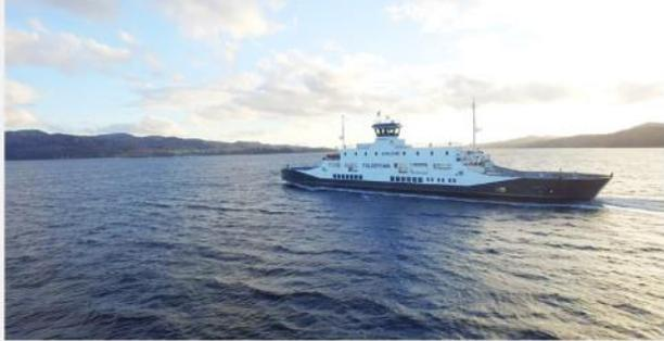
The technology group Wärtsilä has successfully completed a further round of test procedures of its automated dock-to-dock solution. In an unprecedented operation, in the presence of the Norwegian Maritime Authority (NMA), the system was further tested on the ferry 'Folgeforn', this time for full dock-to-dock capability, with the autonomous operation being utilised uninterrupted for the entire route, visiting all three ports serviced by the ship.
