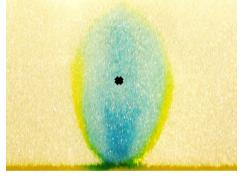
The method developed : 1) Foam injection (yellow) 2) Inject amendment solution (blue)
