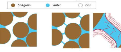
Foam: Gas bubbles separated by water films stabilized by surfactant (lamellea) High viscosity and low density  $\rightarrow$  Better sweeping
