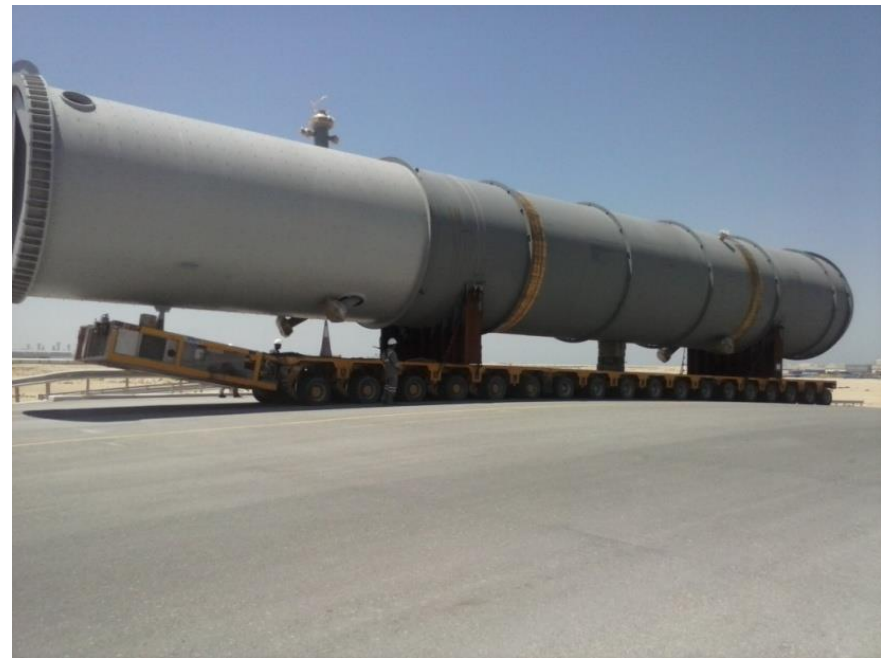
Transportation to site on MSPM
