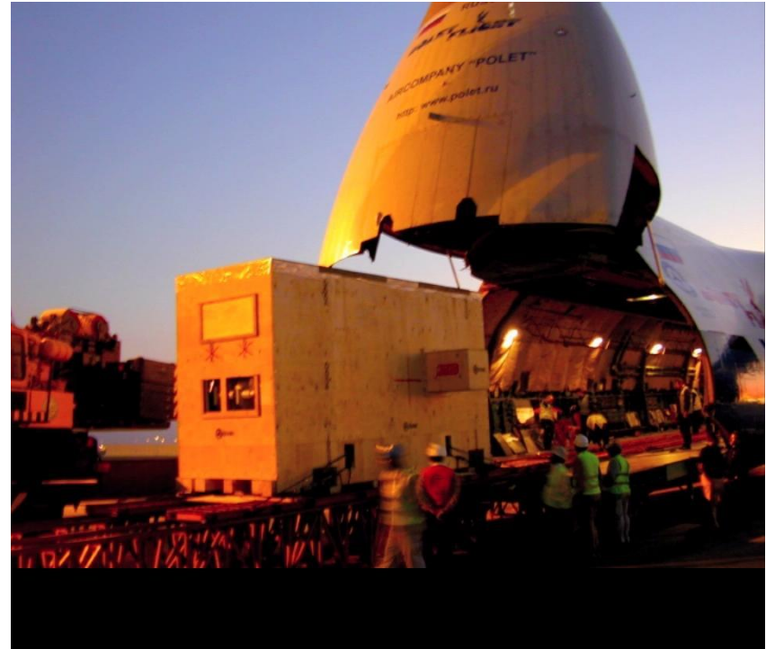
Gear box slowly skid down the tracks laid from inside the aircraft to the tarmac.
