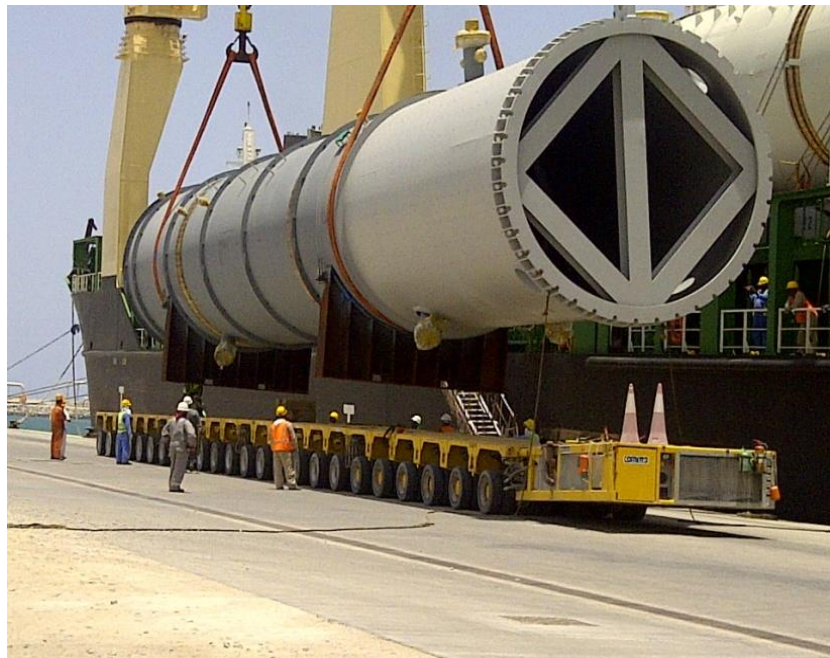
Receiving 36.6 meter long 376.70 Tons HDS Reactor on direct delivery from vessel hook to MSPM
