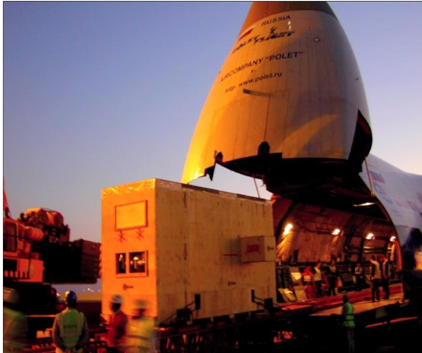
65 Tons gear box being brought out from the cargo flight Antonov at Doha airport.
