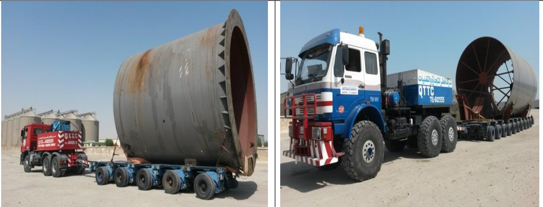
Multi axle trailers with Kiln shells entering site at Umm Bab, Qatar
