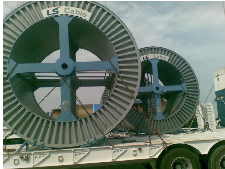
Cable drum lashed on trailer with steel chains.
