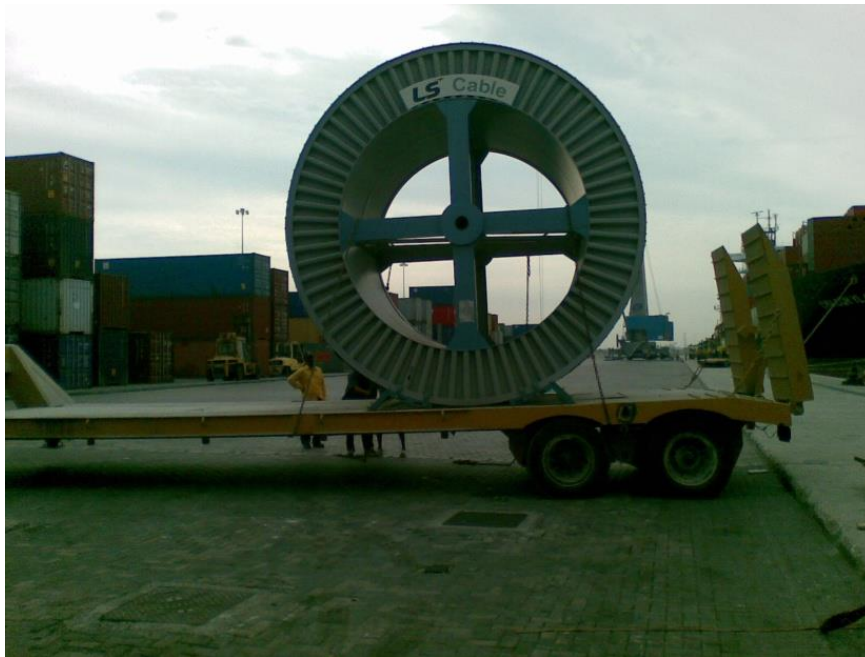
Cable drum on low bed trailer at Doha port.
