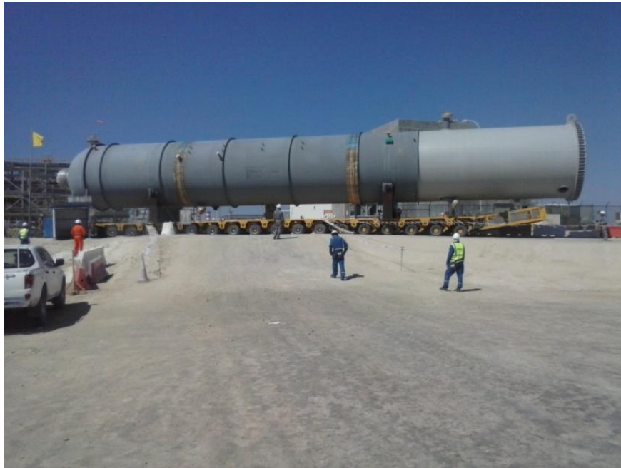
MSPM with HDS Reactor entering site
