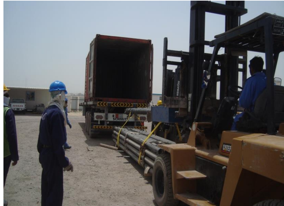
DI pipe bundles being loaded into container
